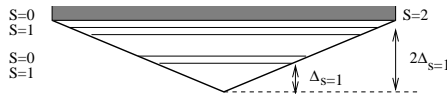
Fig. 5. Singlet and triplet states in the linear potential. The continuum begins at the lowest S = 2 state, E = 2\Delta_{s=1} \sim 4\Delta_{sol} .
